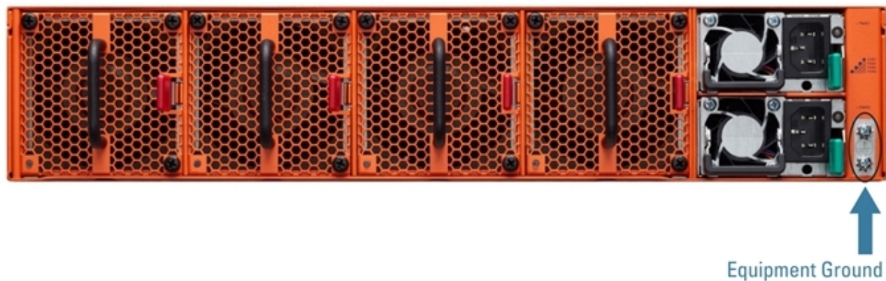
Figure 8 Ground Screws (GigaVUE TA Series-Shown)
